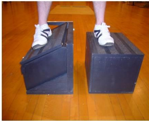
Figure 1. Landing platforms (a) flat, (b) 25°inversion and (c) 25° inversion + 25° plantarflexion surface.
